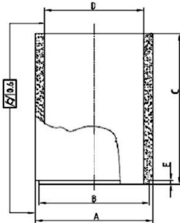
**Filterelement 40 µm**
