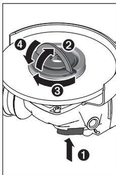
Press the spindle lock button (2) to lock the grinding spindle. To tighten the quick-clamping nut (19), fold up the bar and turn the quick-clamping nut firmly clockwise. Then fold down the bar to secure the quick-clamping nut. **It is not sufficient to tighten the disc along the edge.**
