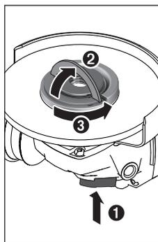
Quick-clamping nuts (19) that are properly secured and not damaged can be removed by hand. To do this, fold up the bar and turn the quick-clamping nut firmly anticlockwise. If the quick-clamping nut is stuck, do not attempt to loosen it with a tool – always use a two-pin spanner.
