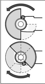
Place the protective guard (10) on the spindle collar. Adjust the position of the protective guard (10) to meet the requirements of the operation. Lock the protective guard (10) by tightening the locking screw (9) using the hex key (4).
