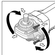
The machine head can be rotated in 90° increments. In this way, the on/off switch can be brought into a more favourable handling position for particular applications, e.g. for left-handed tool users.
