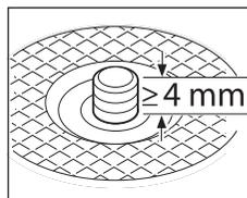
After fitting the hub flange and the grinding/cutting disc, the free thread length of the grinding spindle must be **at least 4 mm**.
