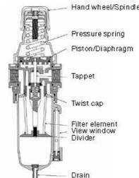
Inspections and maintenance should be carried out regularly after the commissioning. If condensate collects, drain the condensate at brief intervals through the condensate drain plug. The maintenance intervals depend on the operating mode of the filter pressure regulator but should be performed at the latest every 6 months.
